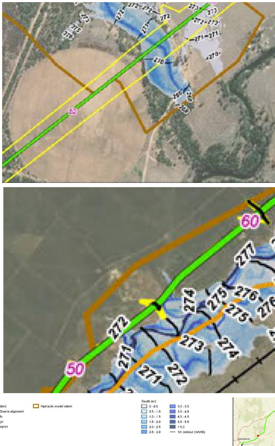
Figure 7-2 - Comparison of Macintyre Brook at Cremascos Road and Macintyre Brook - Yelarbon to Inglewood flood model predicted peak flood extents, levels and depths near Cremascos Road for the 1% AEP event. (from EIS Appendix Q2 Figures J2-E and L2-E)
