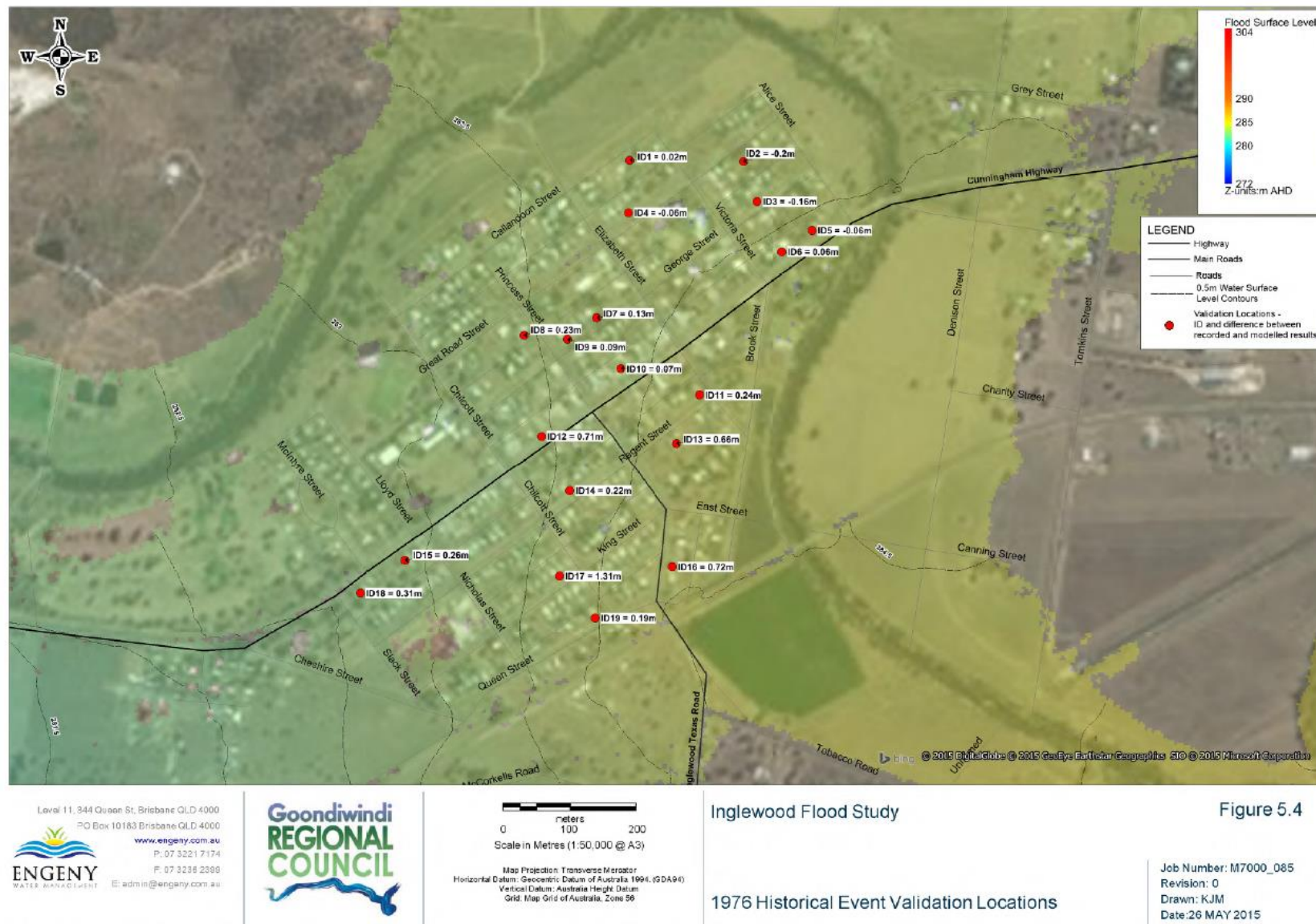
Figure 6-2 - Locations of surveyed 1976 flood peak flood levels (reproduced from Figure 5.5 in Engeny (2015))
