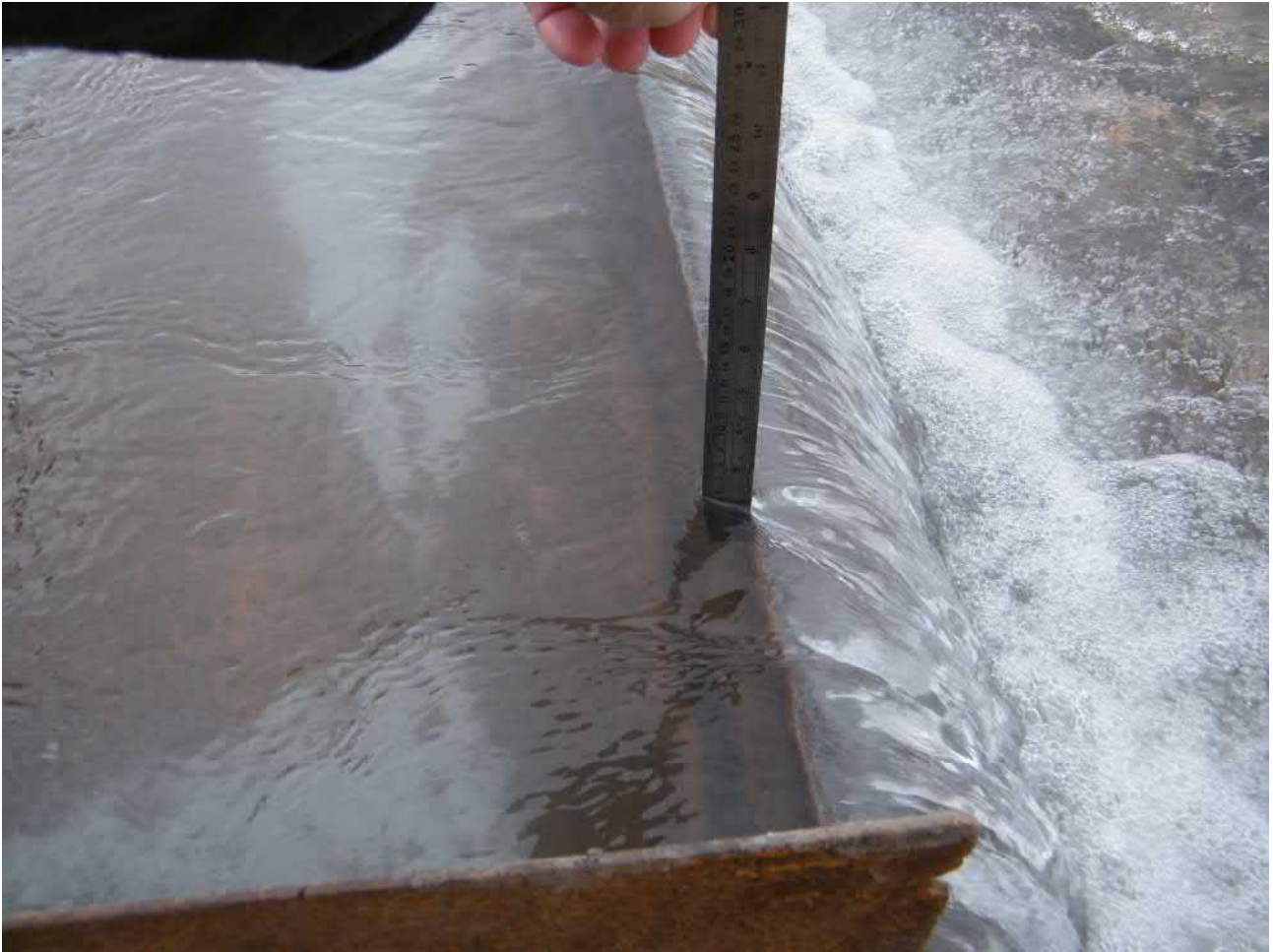
Figure 3 Weir box showing with flow measurement ruler (note sheen on water surface indication of hydrocarbon presence)
