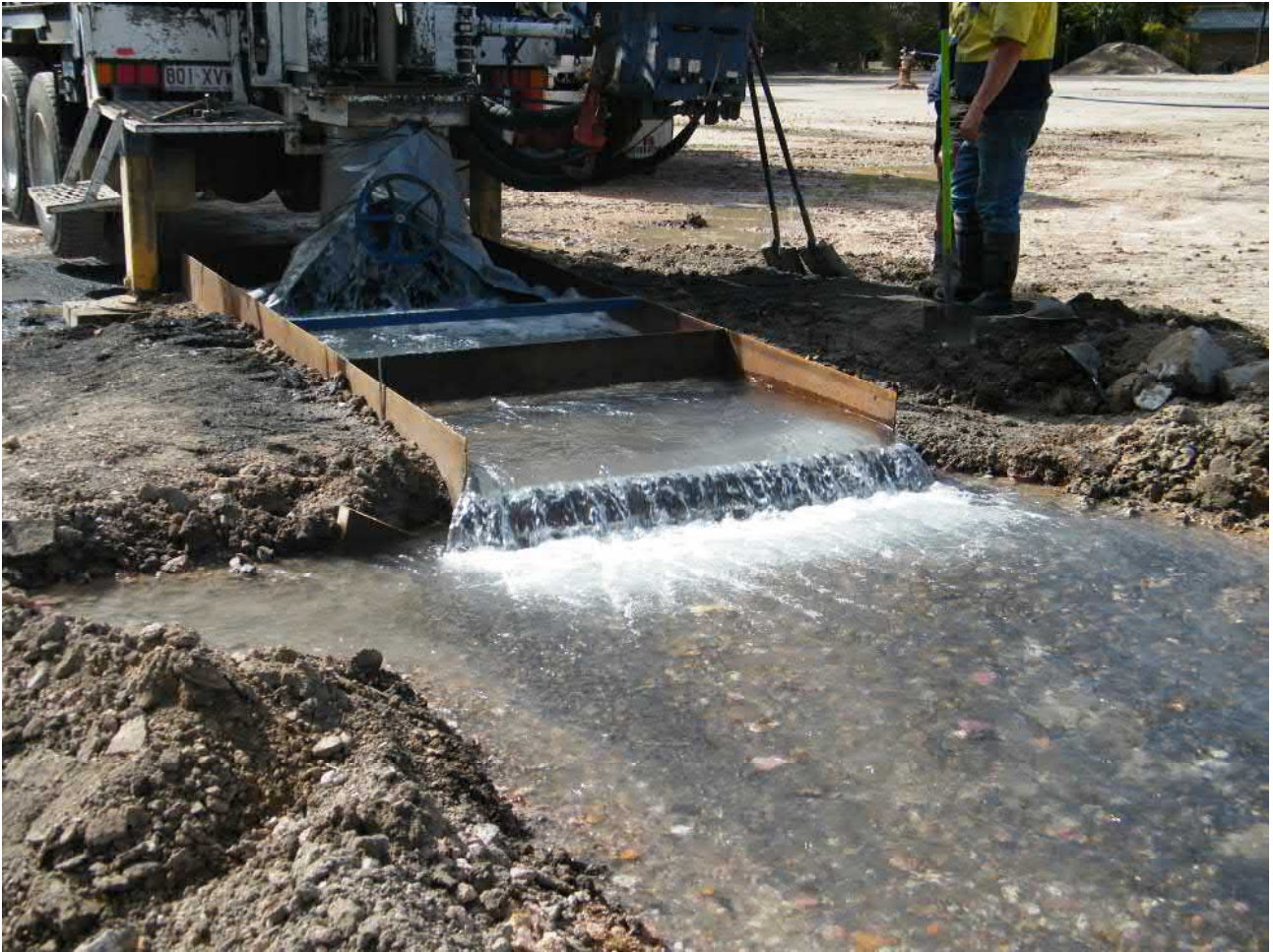
Figure 4 Weir box and earthen channel
