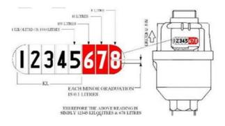
Figure 2: Water meter Diagram
