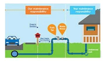
Figure 1: Water meter placement
