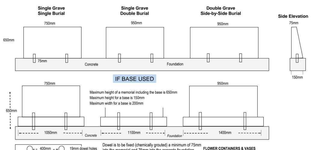
into the memorial and 75mm into the concrete foundation
